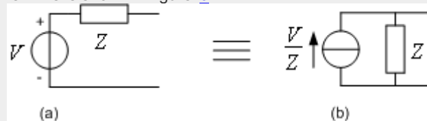
Figure 6: Norton equivalent circuit a) Voltage source in series with an impedance b) Current source representation using Norton equivalent circuit.
